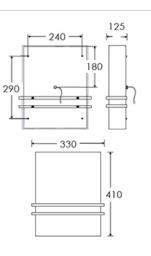
Dimensions in mm and approximate Please note that this fitting requires a cavity / Junction Box with at least 50 mm diameter by 20mm depth to facilitate electrical connection.
