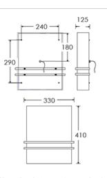
Dimensions in mm and approximate Please note that this fitting requires a cavity / Junction Box with at least 50 mm diameter by 20mm depth to facilitate electrical connection.
