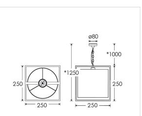
Dimensions in mm and approximate \*Adjustable flex and chain length
