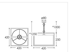
Dimensions in mm and approximate \*Adjustable flex and chain length
